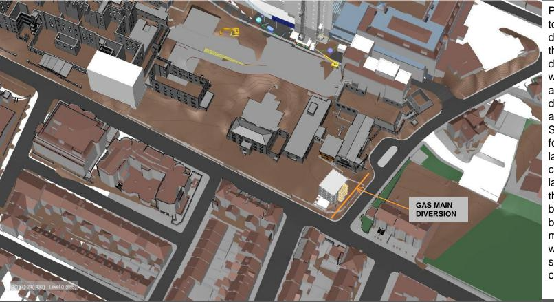
Planned works is to get the gas pipe diversion done at this time so that it does not interfere with the site access at a later date and gives us a head start on the S278 works (new footpath and road layout) that will be completed at a later date. Most of these works will be behind our site boundary. The main connection will be on the south side of the cancer centre.
