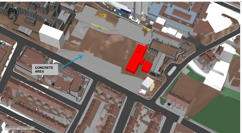
Concrete haul road to be installed, this is to keep delivery vehicles from running on the chalk areas and to keep all delivery vehicles clean before exiting site.
