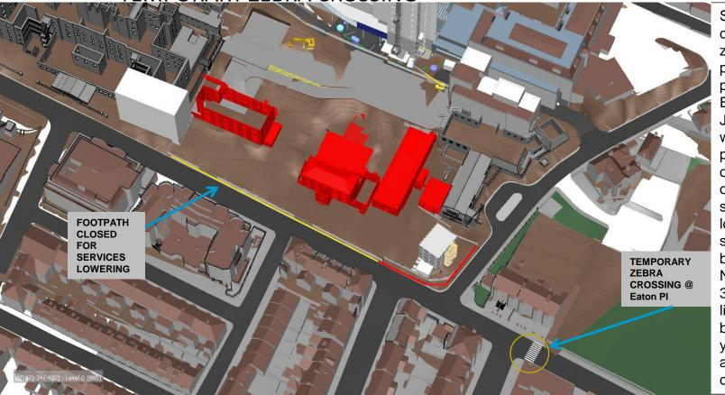
S278 works to commence, new zebra crossing point to be put in place just after the Eaton Place Junction, this is so we can close the pavement in front of the entire length of the site, for services to be lowered and the site boundary to be put in place. New hoarding 300mm from kerb line. This will also benefit the school young children and parents crossing.
