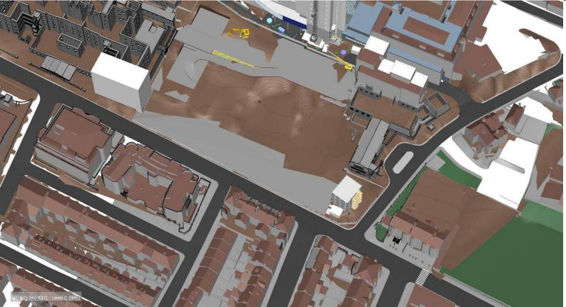
Piling to commence, this will mean that site deliveries will start ramping up. 120 cubic meters of concrete per day. This will equate to 15 TO 20 loads of concrete per day.
