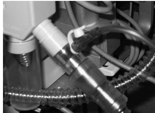
Figure 5. Connecting an external oxygen flow to the expiratory end of the ventilator.
